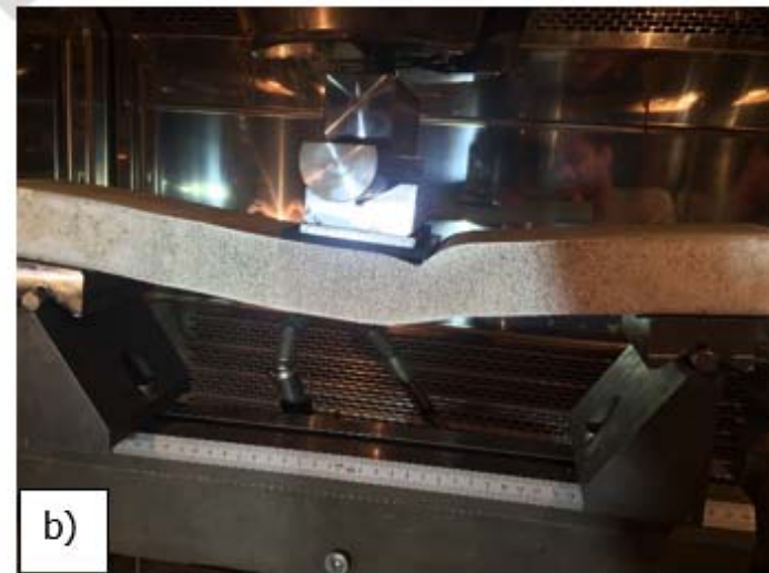
Failure due to a) core shear failure at room temperature b) indentation at elevated temperatures ( 50 °C and above)
