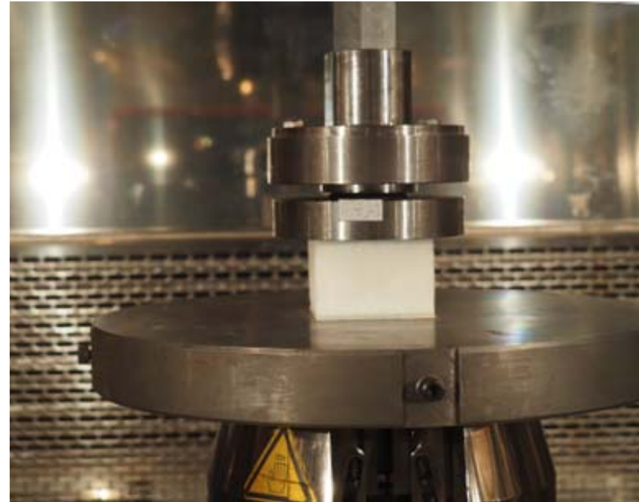
Experimental setup for flatwise compression test of sandwich beams
