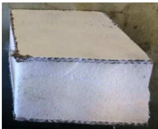
Small scale tests Cone Calorimeter
