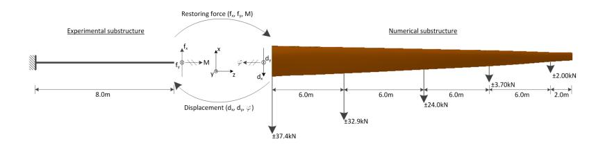
Substructural scale testing of a SSP34m wind turbine blade
