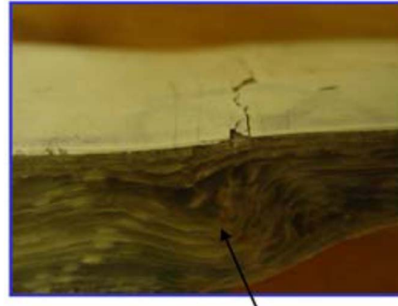
Glass Fiber Reinforced Wind Turbine Blade Local Failure at a Manufacturing Flaw
