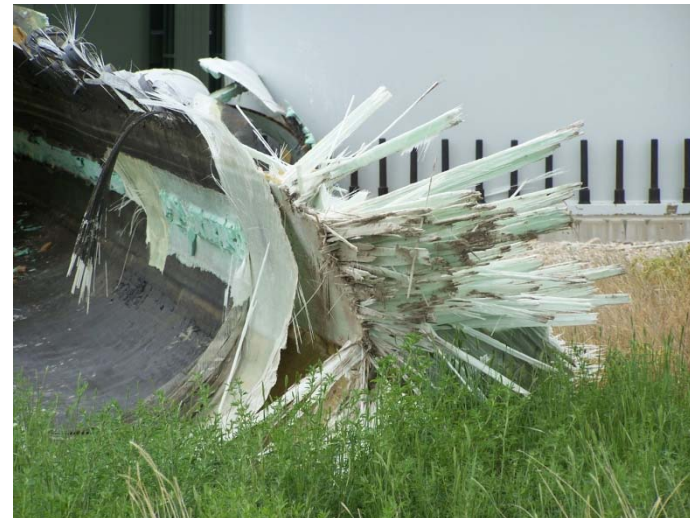
Field Failure of a Wind Turbine Blade (Judith Gap Montana 2009)
