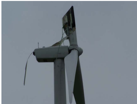
Field Failure of a Wind Turbine Blade (Judith Gap Montana 2009)
