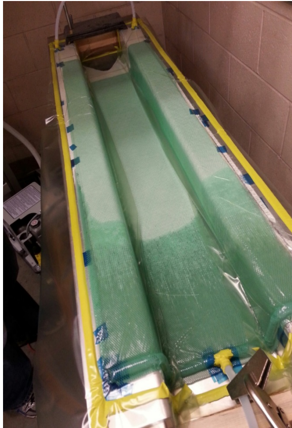
Infusion of Subscale Beams
