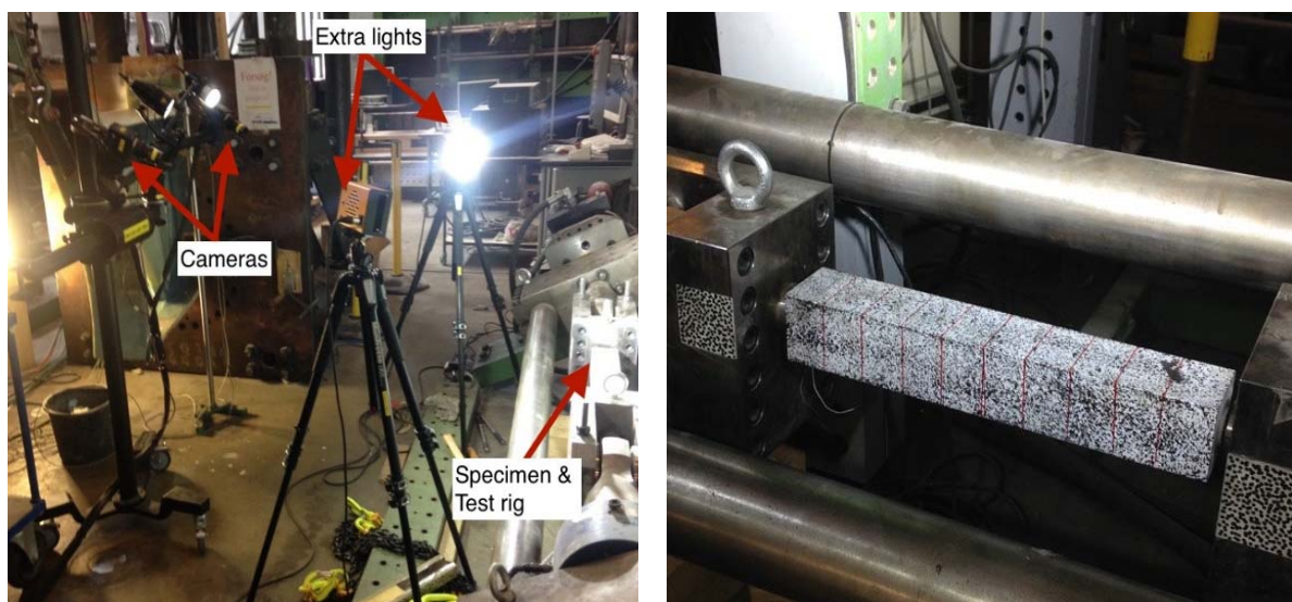
Figure 1. Test set-up for testing of wind turbine root bushing under multiaxial loading
