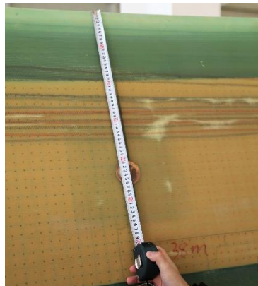
Fig. 4 The whitening of sandwich skins after fatigue test
