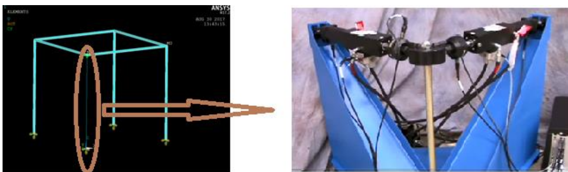
Figure 4, A hybrid test system with one column being tested
