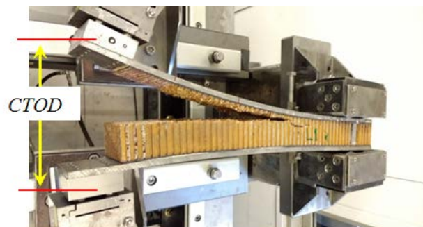
Figure 7. Crack tip opening displacement (CTOD) measurement.
