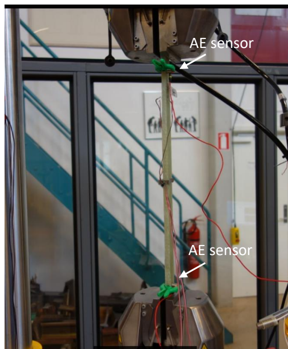
Figure 4: Location of the acoustic emission (AE) sensors for static and fatigue tests.
