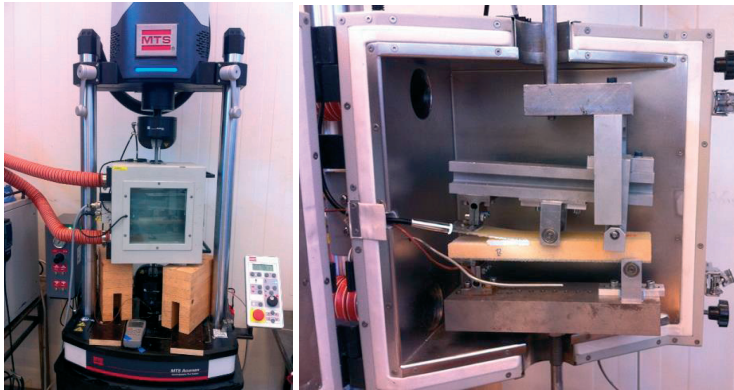
Figure 1: Sandwich MMB test setup inside climatic chamber
