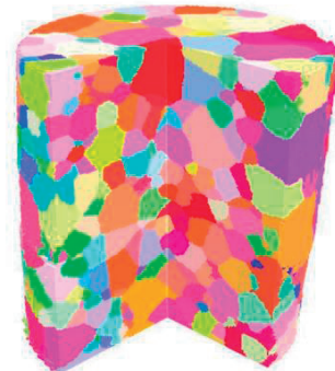
LabDCT reconstruction of the grain structure in a cylindrical Fe sample with a diameter of 1 mm.
