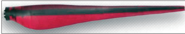
Figure 3: Blade with carbon-fibre spars where fibers are biased to the blade pitch axis to introduce bend-twist coupling.
